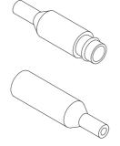
The male IP172 interconnection protector should be assembled on a TQxxx proximity sensor's integral cable.
